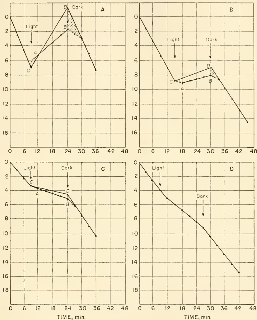
Fig. 29.4. Quantum yield measurements with Chlorella (after Warburg 1948). Yellow light, 10°C. Shaded areas represent "induction losses" attributed to sluggishness of manometer. (Curve A shows a slight excess instead of deficiency of gas evolution at the beginning of illumination.) Quantum yield is determined from difference between slope in light ( AB or CD , depending on the method of calculation) and slope in darkness.
